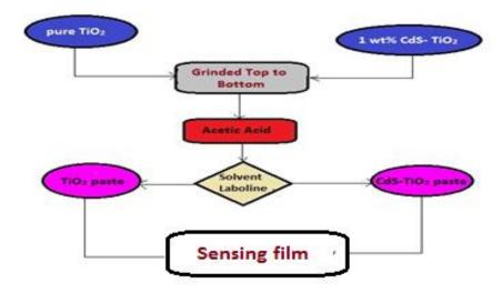
Figure 1. Flow Chart of Fabrication of Film
