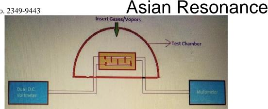
Figure 3. Experimental Setup for Sensing of LPG
